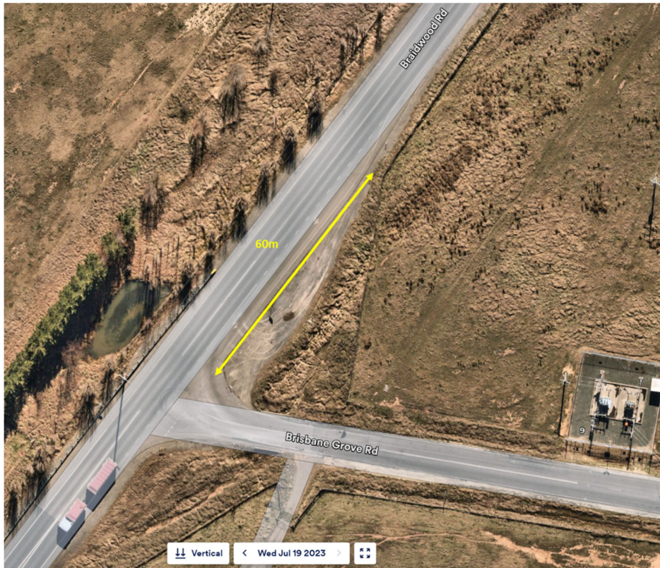
Figure 2 – Existing BAL Intersection Arrangements of Brisbane Grove Road / Braidwood Road
